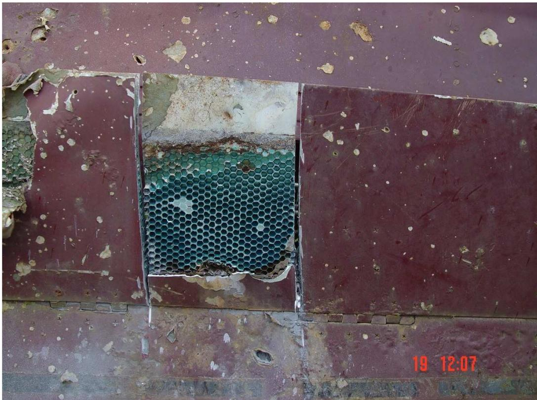
**Fig. 27: Rear Section Left Wing – Sectioned (1)**
