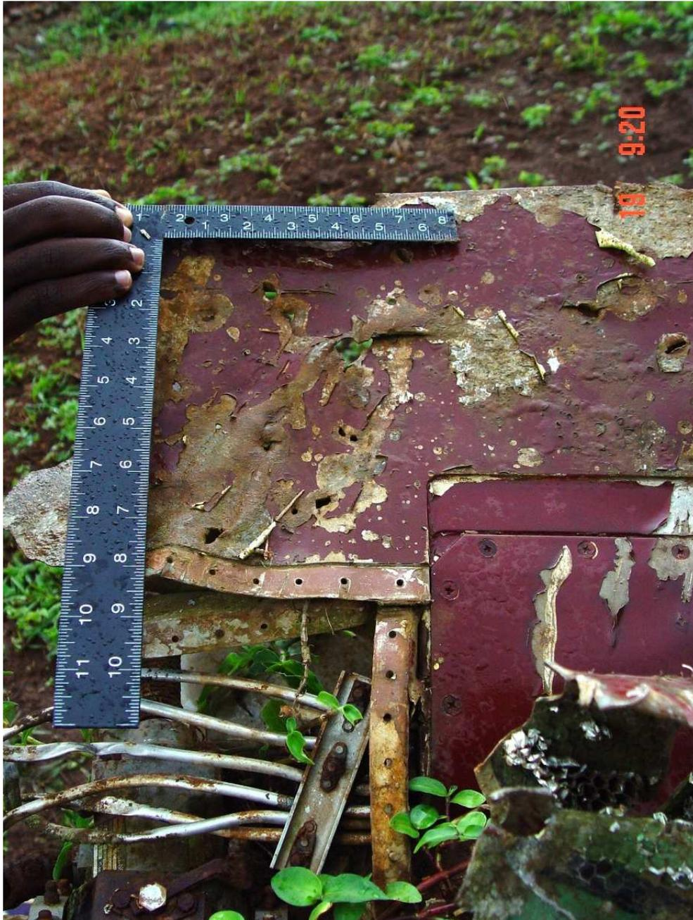
Fig. 23: Rear Section of Left Wing (2).
