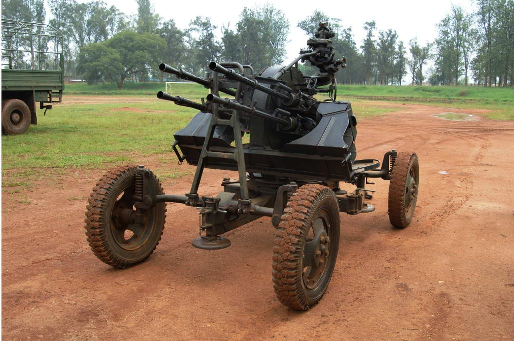
**Fig. 17: View of 14.5mm Anti Aircraft Gun (Quad Mount).**
