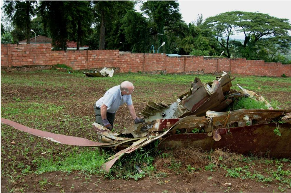
**Fig.10: Right Wing and Rear Section of Left Wing (1).**
