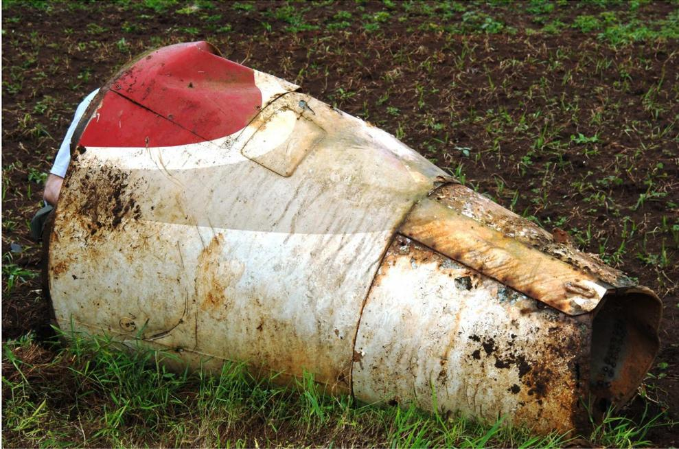
**Fig. 20: Tail Exhaust Cone.**
